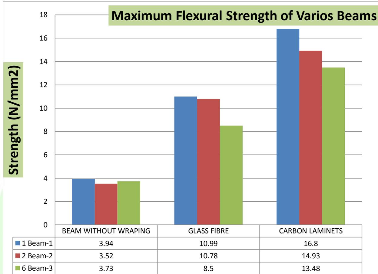
Figure-2: Graph for maximum flexural strength (N/mm<sup>2</sup>)
