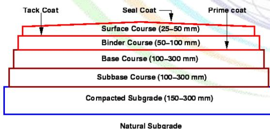
**Fig-2: Flexible pavement design**
