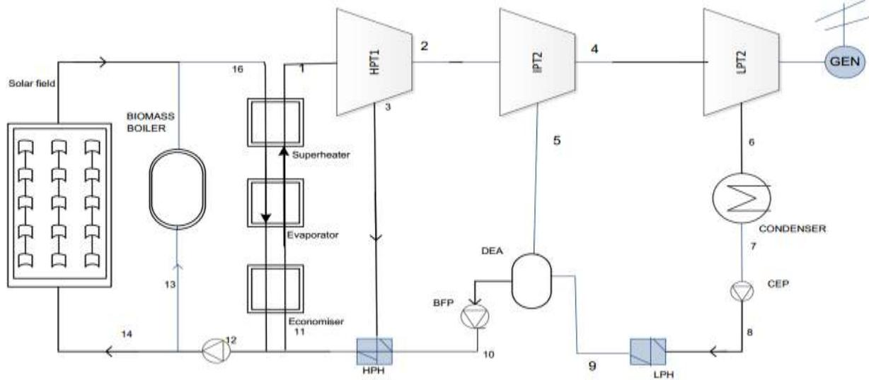
Fig. 1. Solar-Biomass hybrid power plant
