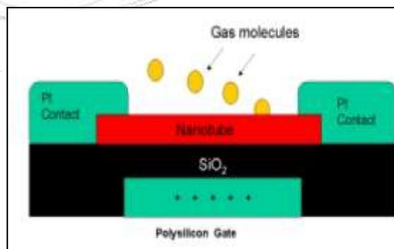
**Fig. 2: Nanotube based Chemical Sensor**
