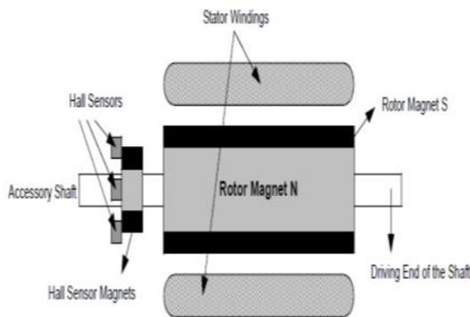
Fig. 1. Cross section view of BLDC Motor
