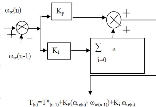
Fig. 4 Basic structure of PI controller
