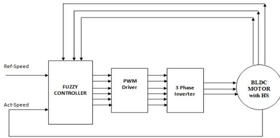
Fig. 8. Block Diagram of Fuzzy Controlled BLDC Motor Drive
