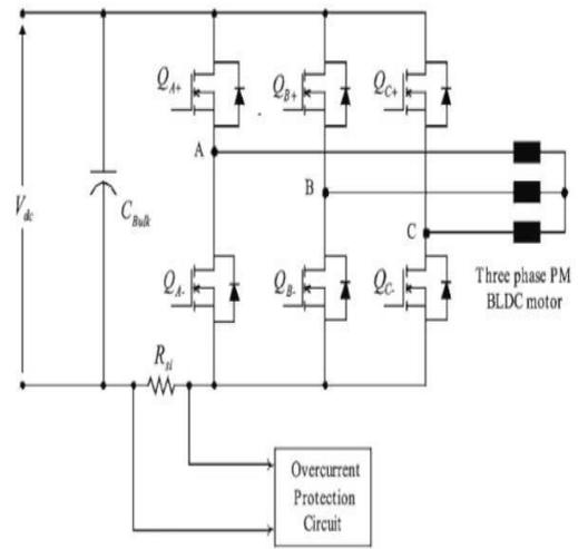
Fig. 2. Three-phase MOSFET inverter driven BLDC motor
