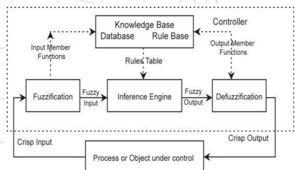
Fig. 7. Basic block diagram of FLC
