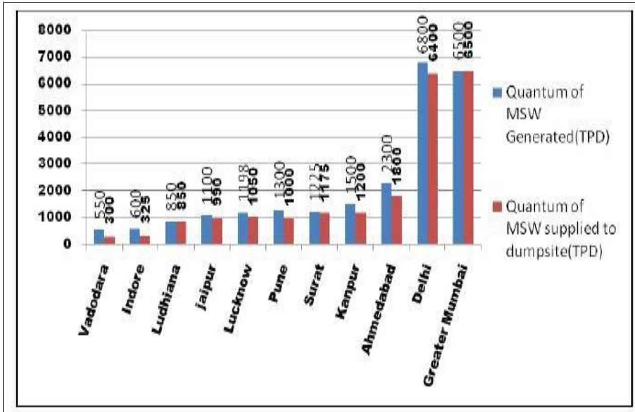
**Figure No-2:** Bar graph representing the quantum of waste generated and the Quantum of waste supplied to the dumpsite for Cities generating more than 550 TPD.
