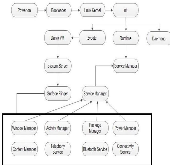
**Figure 3: Android Bootup Process**
