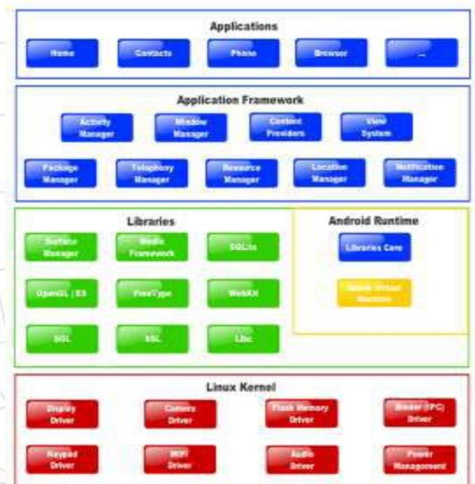
Figure 2: Architecture of Android
