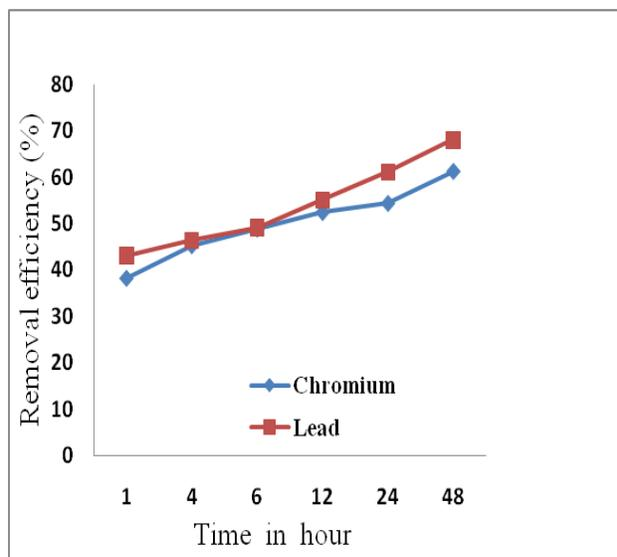
Fig 5: Effect of EDTA (0.01M) on removal of Pb and Cr.
