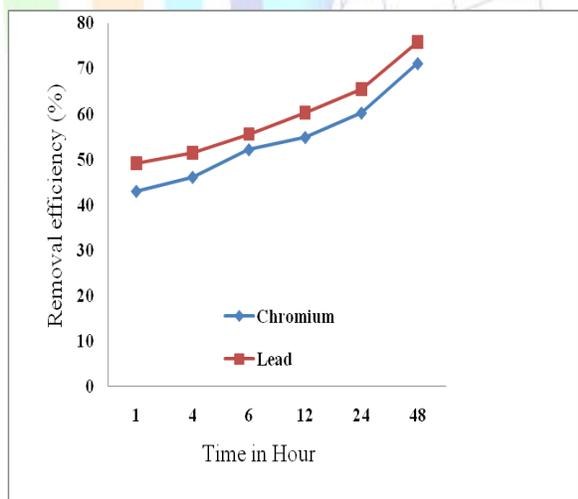
Fig 6: Effect of EDTA (0.05M) on removal of Pb and Cr
