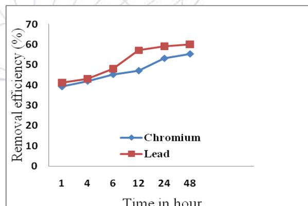
Fig 4: Effect of EDTA (0.005M) on Removal of Pb and Cr.
