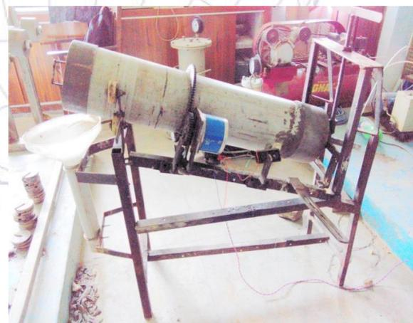
Fig 2: Bench Scale Model for Soil Washing
