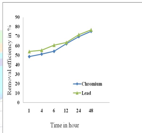
Fig 7: Effect of EDTA (0.1M) on removal of Pb and Cr.
