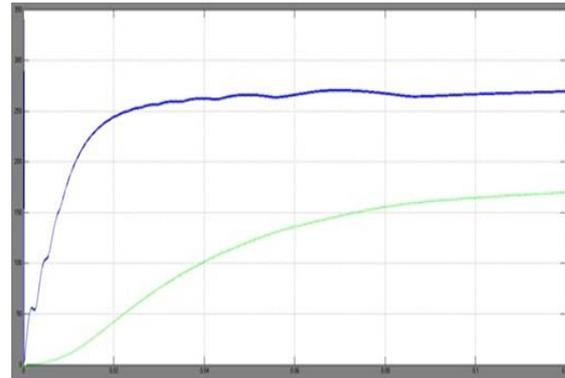
**Fig13. Solar output power without MPPT controller and buck-boost converter and output power with MPPT controller having buck-boost converter.**
