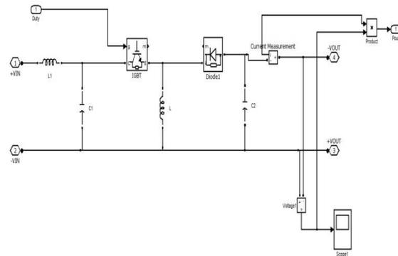
**Fig5.Simulink model of buck-boost converter**
