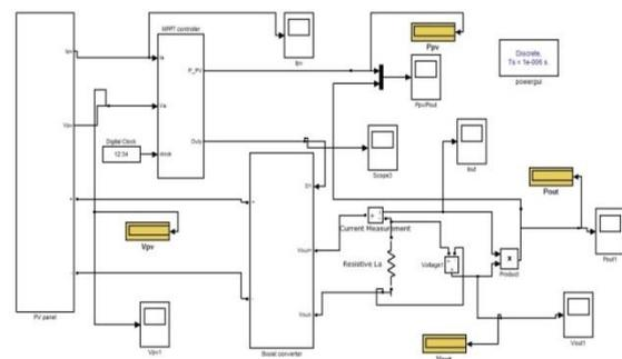
**Fig6.Simulink model of solar panel system using boost converter**
