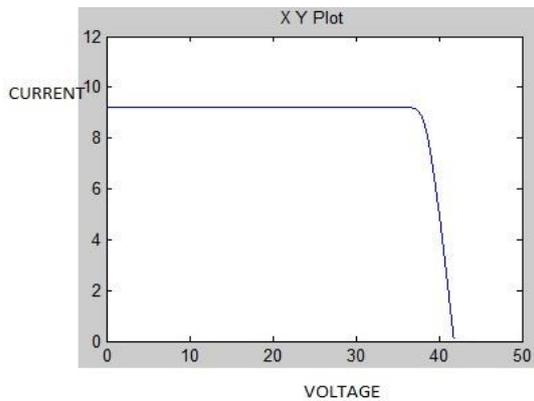
**Fig9. I-V characteristics of a PV module**
