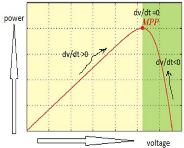
**Fig2.Photovoltaic output power and photovoltaic output power derivative in function of the output voltage**
