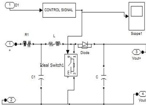
**Fig4. Boost converter Simulink model**
