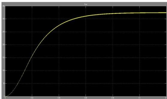
**Fig11. Output power with MPPT controller and boost converter**
