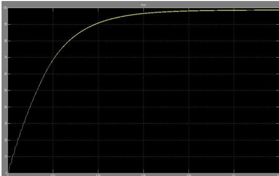
**Fig10. PV output voltage with MPPT controller and boost converter**
