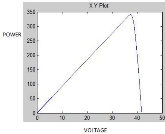
**Fig8. P-V characteristics of a PV module**
