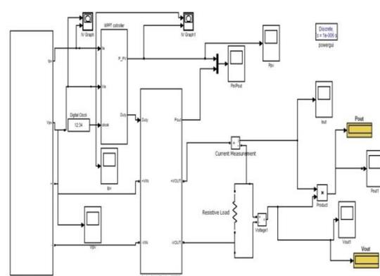
**Fig7.Simulink model of solar system using buck-boost converter and MPPT converter**
