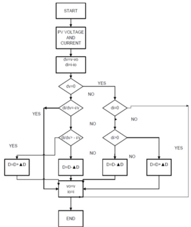
**Fig3.Flowchart for Incremental conductance algorithms for MPPT controller**
