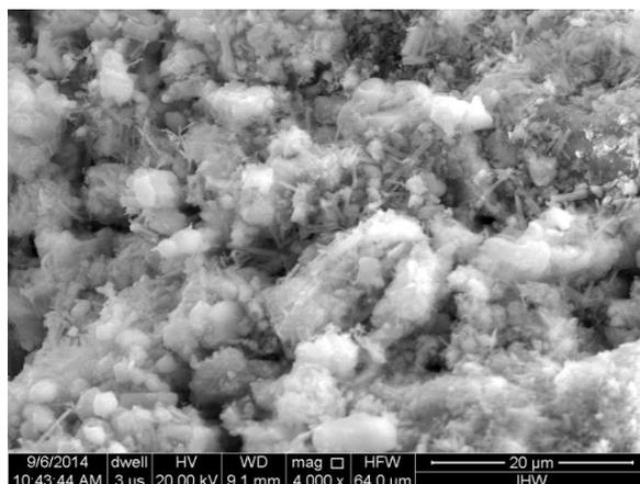
**Figure 6; SEM Image of IHW+9%Lime at 4000X magnification**
