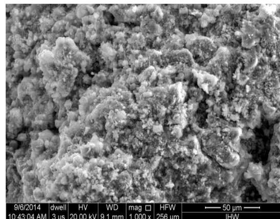
Figure 5; SEM Image of IHW+9%Lime at 1000X magnification
