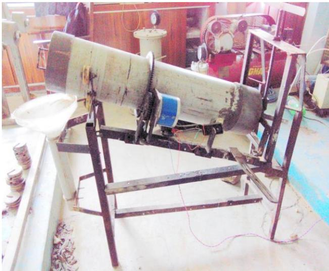
**Fig 2: Bench scale model for the soil washing process**
