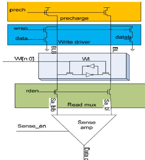
Figure 1: Basic schematic of one column for small signal memory array using 6T cell
