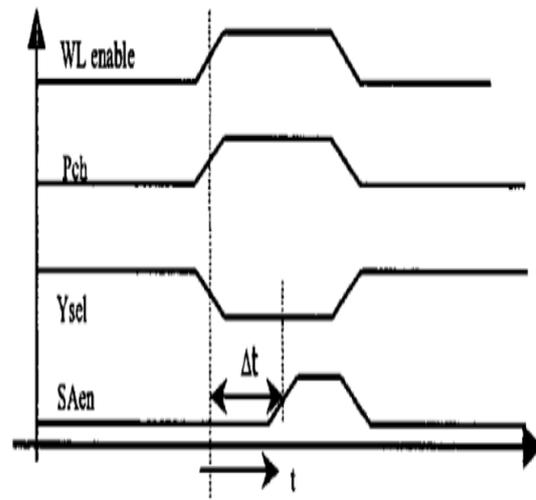
Figure 3: Timing Scheme for a Voltage Sense Amplifier
