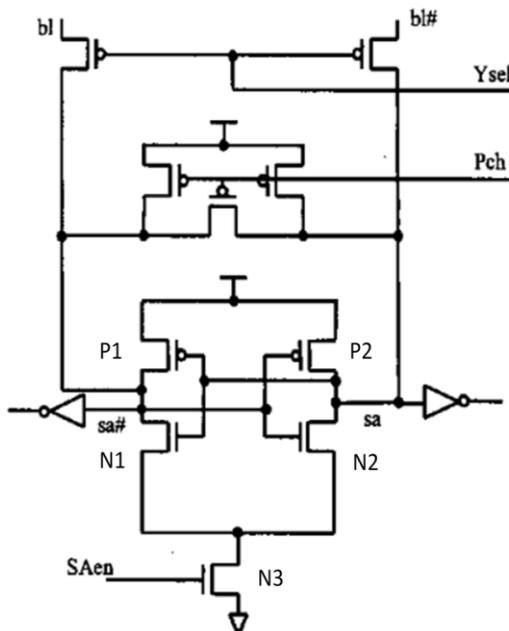
Figure 2: Voltage Sense Amplifier
