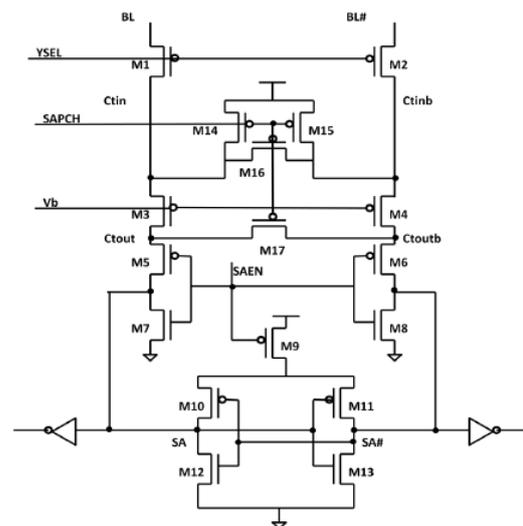
Figure 6: Charge Transfer Sense Amplifier
