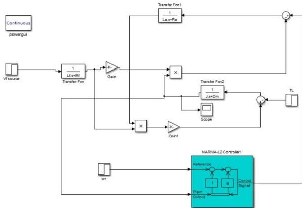
Fig(3) Simulink model of speed control of dc motor using NARMA L2 controller
