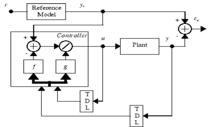
Fig (2): Block diagram of NARMA L2 Controller
