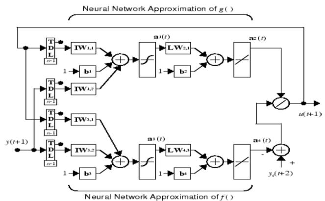
**Simulink Model of NARMA L2 controlled separately excited dc motor:**
