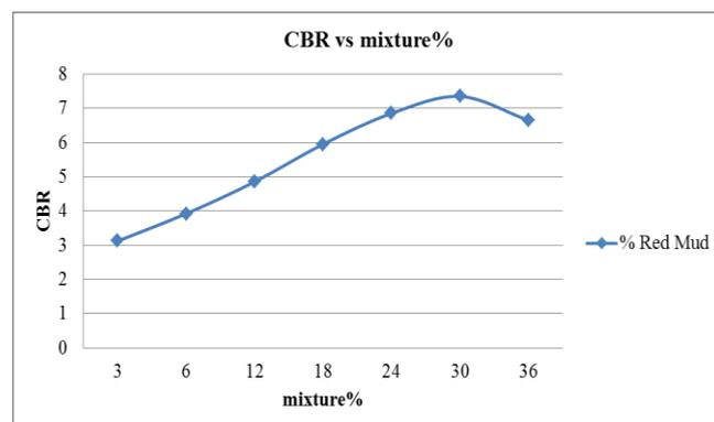
**Fig. 1 % of mixture and CBR curve**
