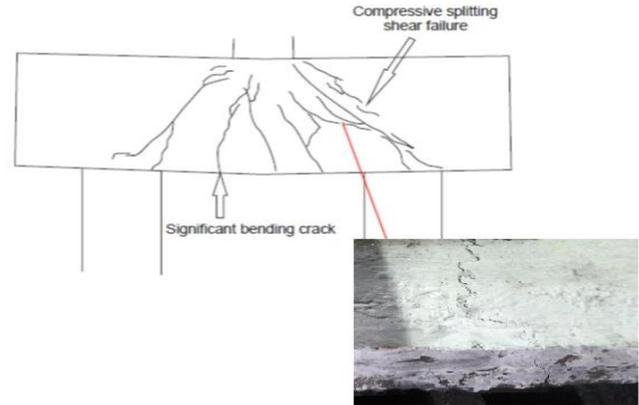
**Figure-9 Crack distribution on PC-2A front surface at failure step**
