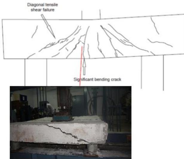
**Figure-7 Crack distribution on PC-1B back surface at failure step**
