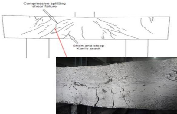
**Figure-3 Crack distribution on PC-2B back surface at failure step**
