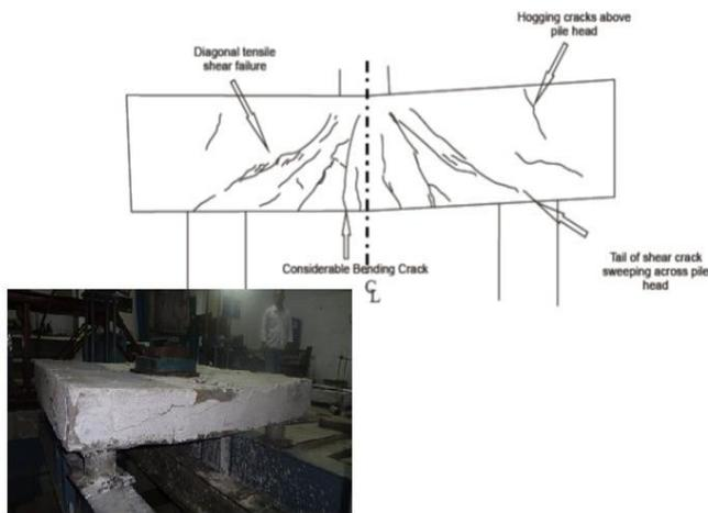
Figure-10 Observed crack pattern
