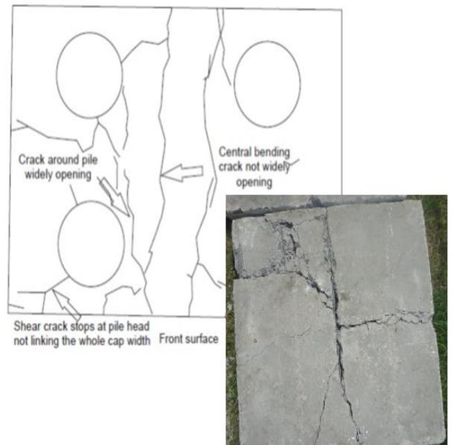
**Figure-6 Crack distribution on PC-1C cap soffit at failure step**
