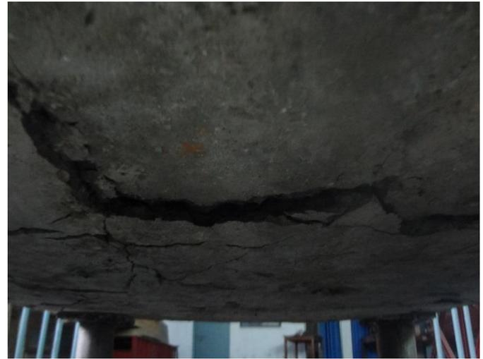
Figure-12 Observed crack pattern in experiment
