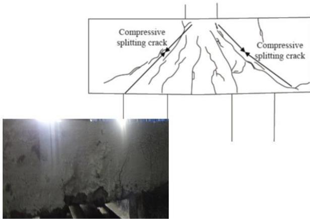
Figure-11 Crack distribution from experiment at the onset of the yield stage
