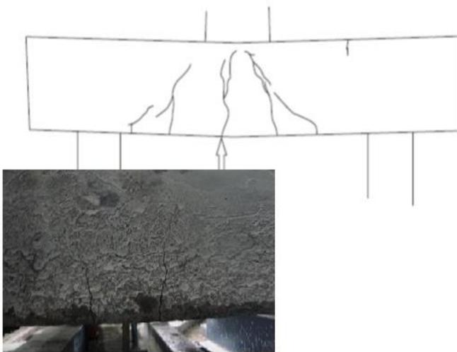
**Figure-8 Crack distribution on PC-2C back surface at failure step**
