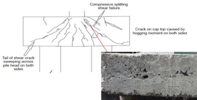
**Concrete being crushed under vertical loading**
