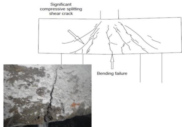
**Figure-10 Crack distribution on PC-3C back surface at failure step**
