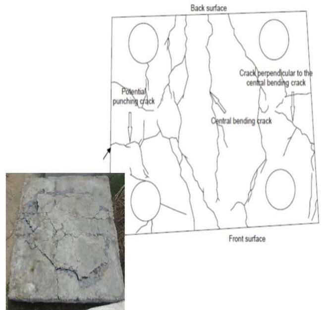
**Figure-5 Crack distribution on PC-1A cap soffit at failure step**
