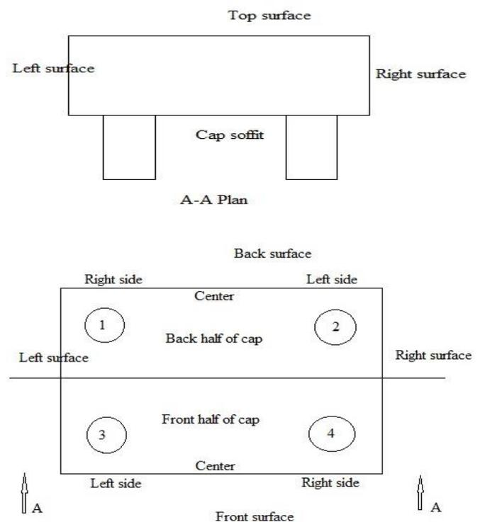
Figure-1 Terminologies for describing the crack distribution and propagation
