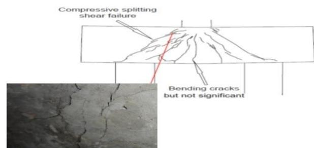
**Concrete being crushed under vertical loading****Figure-2 Crack distribution on PC-3A front surface at failure step**
