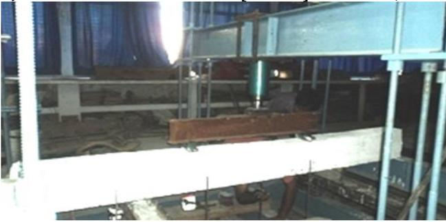
Figure 4. Spreader I- Beam Used To Perform 2 Point Loading
