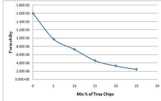
Fig. 3 permeability vs. mix% of tire chips
