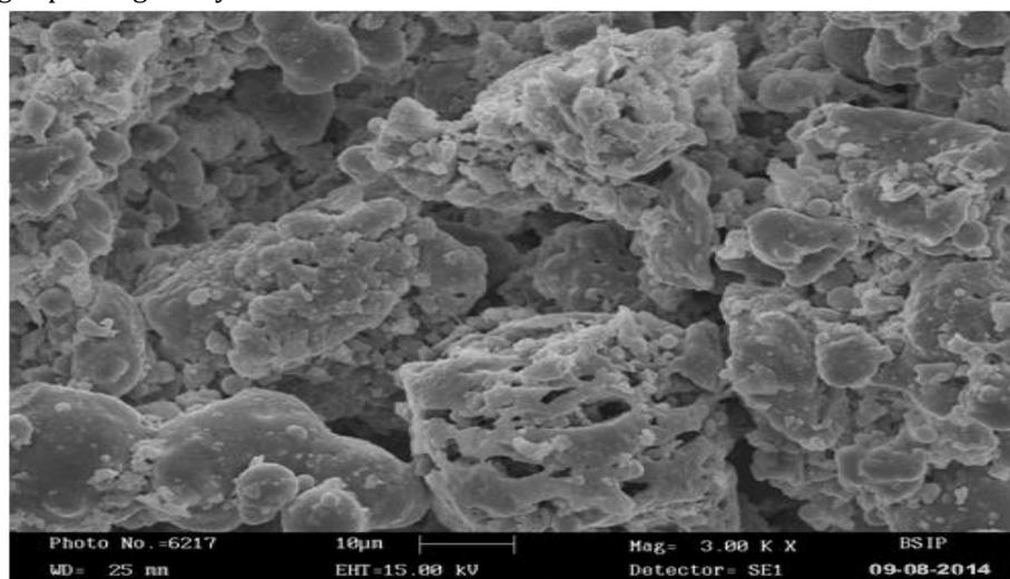
**Fig. 3: SEM image of 60% soil +38% flyash +2% geofiber at 3000X magnification**
