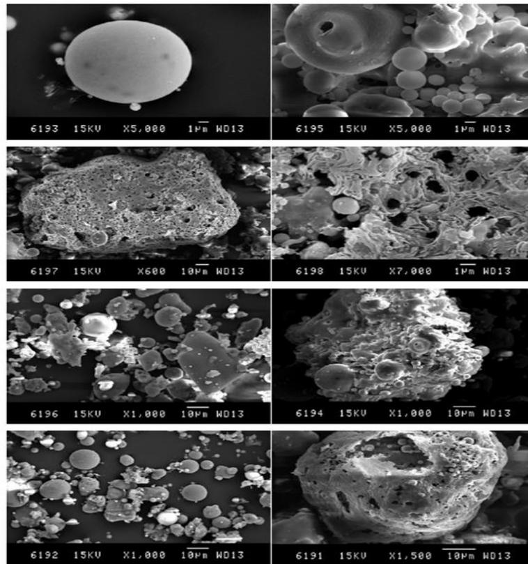
**Fig. 2: SEM image of Fly ash at different magnifications (Source NTPC Tanda)**
