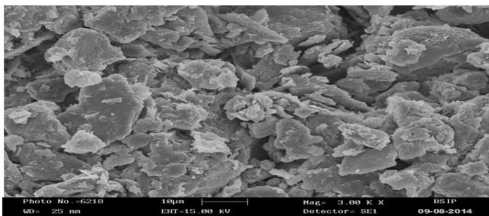
**Fig. 4.1: SEM image of Soil AT 3000X magnification**
