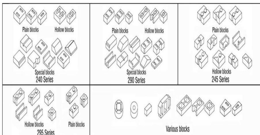
**Fig. 1** Different types of compressed earth blocks
